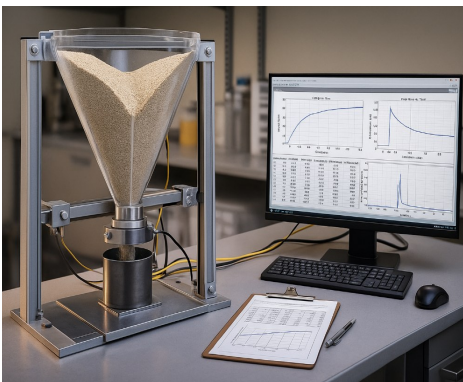
Flow Through Orifice analysis set-up
