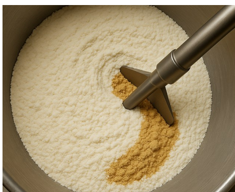
Non-homogenous powder mixture in a mixer.
